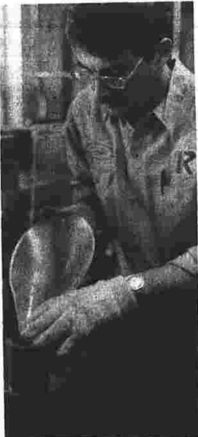
DAVID WRIGHT POURS PLASTIC INTO MOLD ... to be compressed into a solid disc.
